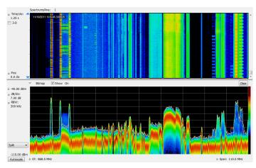
DPX Spectrograms (Opt. 200) provide gap-free spectral monitoring for up to days at a time. 60,000 traces can be recorded and reviewed, with resolution per line adjustable from  $110~\mu s$  to 6400~s.
