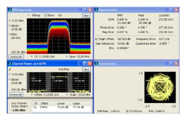
Time-correlated, multidomain views provide a new level of insight into design or operational problems not possible with conventional analysis solutions. Here, ACLR and Vector Modulation Quality (Opt. 21) are performed on a single acquisition, combined with the continuous monitoring of the DPX® spectrum display.
