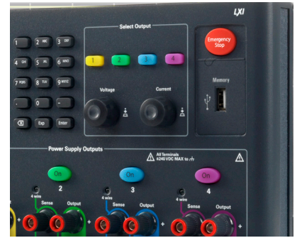
Figure 11. The N6705's front panel USB port.
