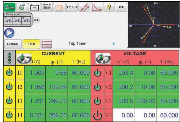
Figure 2. Manual Test Screen – 4 Channel Unit
